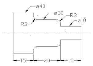
4. Make the following job of aluminium billet of  $\phi$  30 mm & 60 mm long using turning operation on CNC machine
