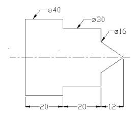
3. Make the following job of aluminium billet of  $\phi$  40 mm & 70 mm long using turning
