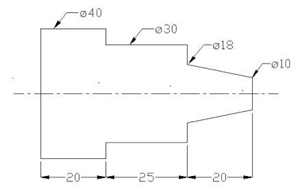
2. Make the following job of aluminium billet of  $\phi$  40 mm & 70 mm long using turning operation on CNC machine.
